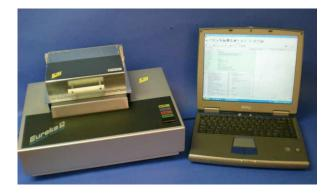
The CST new **"ABT" Heat Chamber Box System** provides a unique and costeffective approach to testing memory modules up to 80 Degree C. This compact system is ideal for "bench top" applications and includes an integrated thermal heater box using – Halogen Lamp technology for rapid heat ramp-up and precision temperature control for Heat and Cool down.
